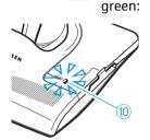
If the operating mode was changed successfully, the charging indicator for the spare rechargeable battery 10 goes off and the indicator (14) lights up again.
